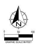
All bearings shown are based on grid north of the Texas Coordinate System of 1983, North Central Zone (4202), North American Datum of 1983.
